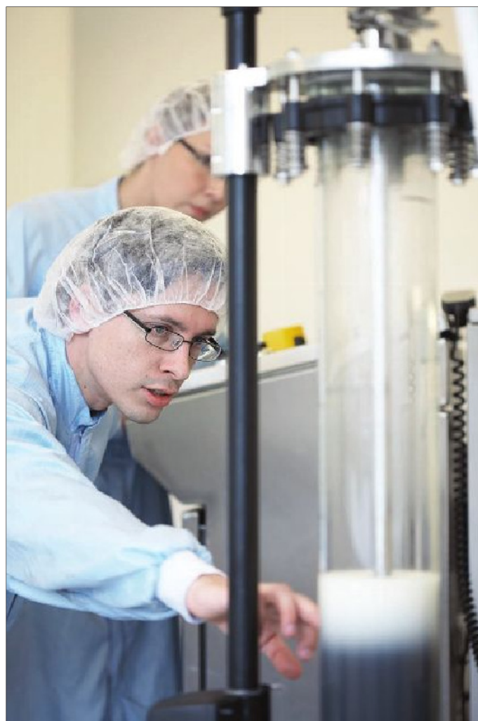
Fig. 1. EBA eliminates pre-treatment of the whey and ensures high capacity and fast flow rate.
